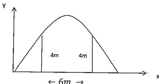
If  $\alpha = 45^\circ$  and the ball just clears two vertical posts, which are both 4 metres above the level of projection and 6 metres apart, calculate the range,  $R$ . 3
